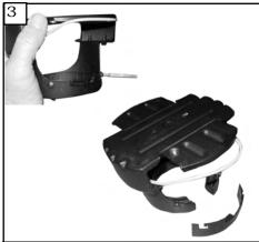
Remove Safety bar from mounting bracket by loosing screws, sliding bar to side, and lifting it off the 2 screws.
